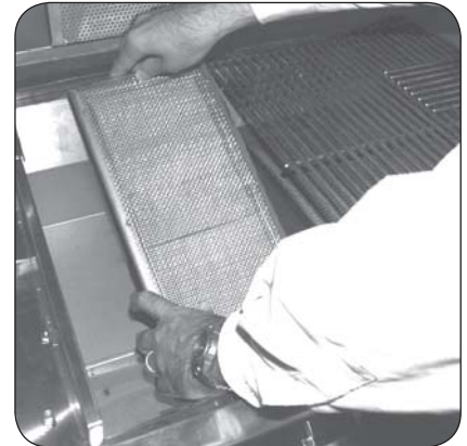
Fig. 4-3 Install new burner
