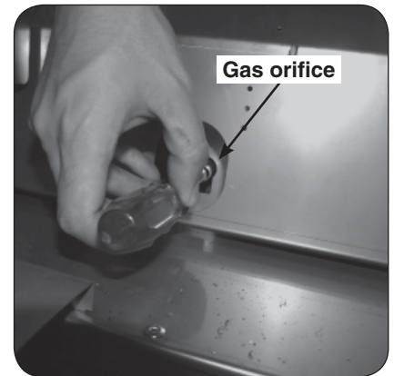
Fig. 3-2 Replace the gas orifice
